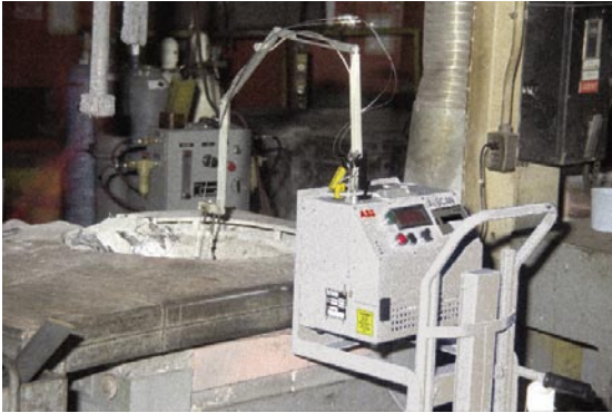
Optional elongated probe arm Courtesy of GM Central Foundry
